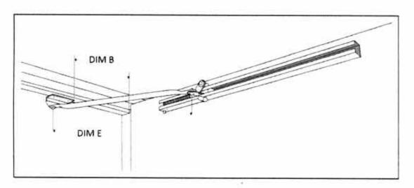
1 : POSITION THE CHANNEL ON THE DOOR FACE, WITH THE DOOR CLOSED INTO THE FRAME.
